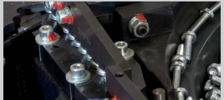
*Detail: exit track with hinged cover tail for rapid fault clearance*
